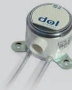
DOL 18 is a negative-pressure sensor that measures the pressure difference between inside and outside air. It emits a 0-10 V signal. Power for this sensor is supplied by ViperTouch.
