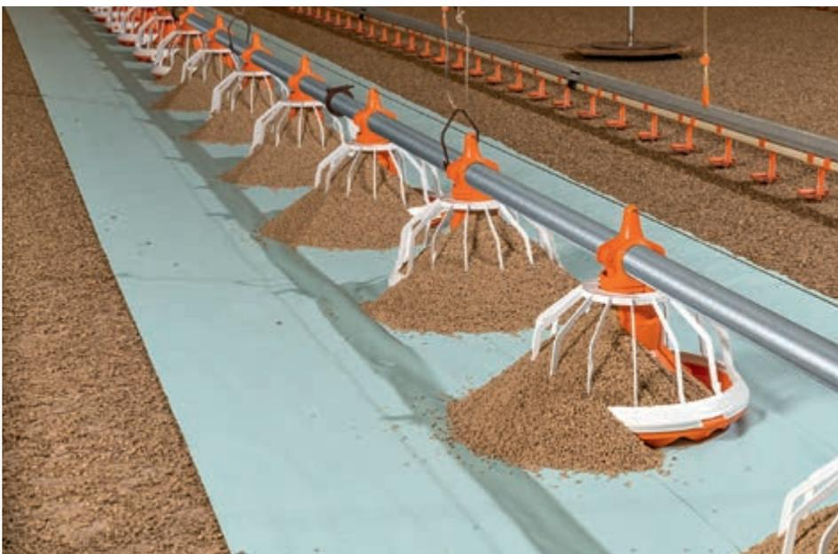
The specifically developed FLUXX 330 feed pan can be overfilled for an ideal chick start
