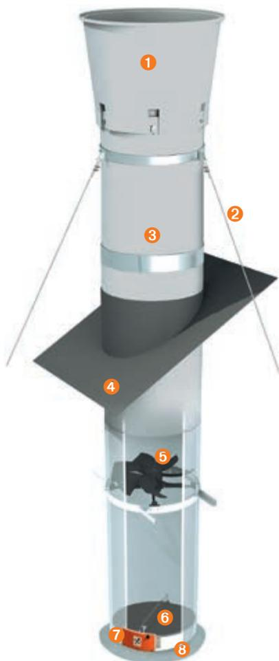
The TopSeal roof covering is an alternative to the roof sheet. This roof covering is made of a black, weather- and UV-resistant EPDM film (special rubber), which is permanently elastic and highly tear-proof and therefore has a long service life. TopSeal is delivered pre-assembled and includes a collar based on the chimney diameter. This makes assembly on site quick and easy. TopSeal can be used for roofs with a slope of up to 20°.
