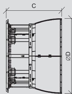
The fan must be equipped with a wire mesh guard in front of the shutter where it is installed at a height of less than 2.70 m and accessible by people.
