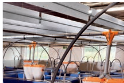
Twin pipe: less dust on pipes
