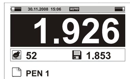
The memory symbol flashes on the display until the weight is removed and logs the last weight saved on the display beside the memory symbol.
