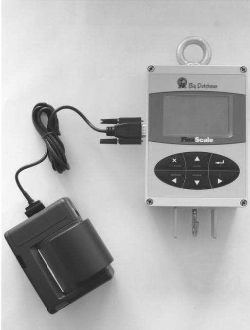
Connect the printer cable into the DB9 serial port on the scale and switch the printer on.
