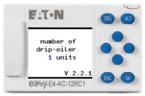
Figure 5-1: Input of number of drip oilers
