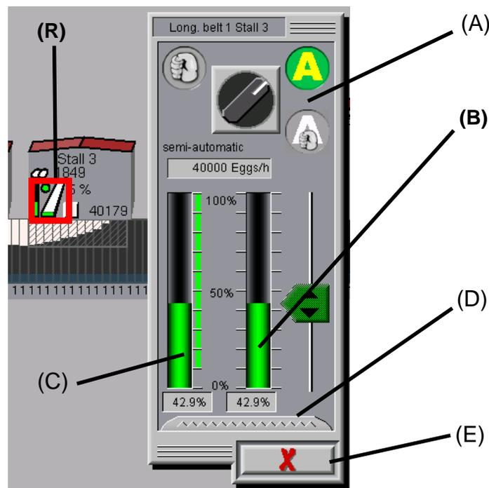
Figure 3-10: Longitudinal belt in automatic mode
