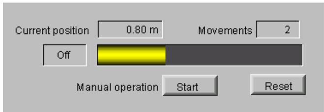
If egg collection is cancelled or a cycle is completed, the values "Current position" and "Movements" are reset.
