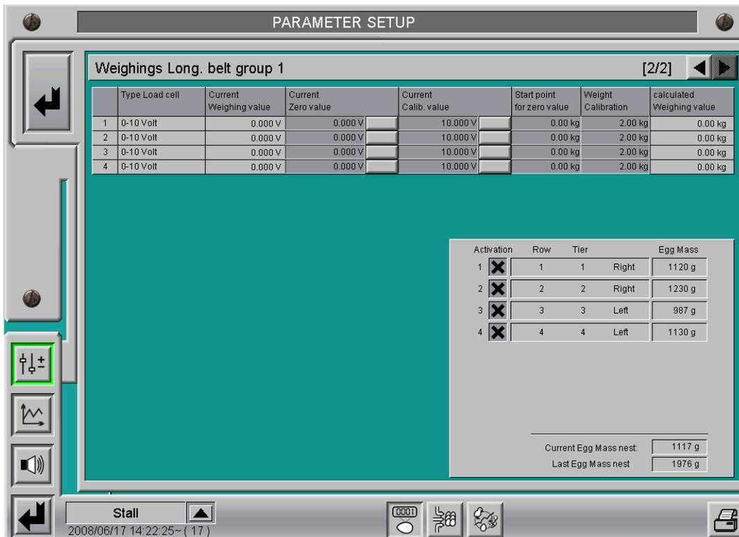
Figure 7-7: Weighing units
