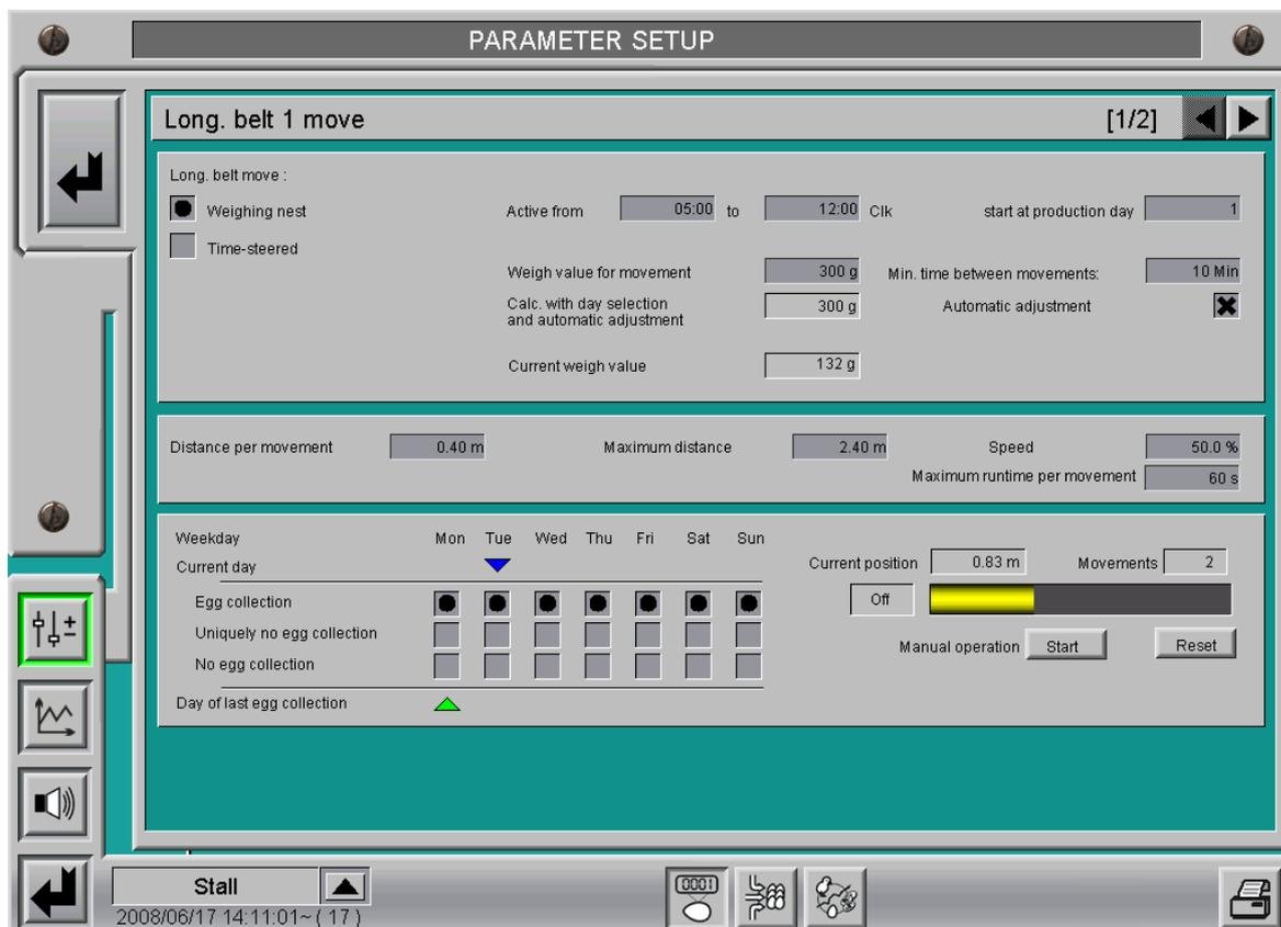
Figure 7-2: Settings: weighing or time-controlled
