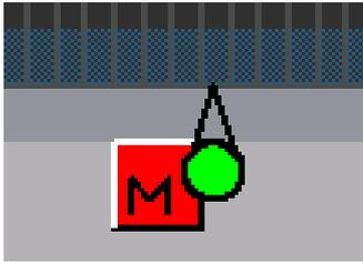
If a motor alarm is configured for a belt control, it is displayed as an alarm message. In addition, the alarm for the particular belt control is displayed on the cross belt.
