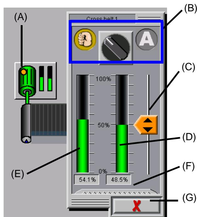
Figure 3-9: Manual operation of the cross belt
