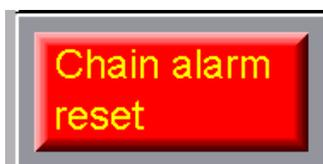
If the chain crack alarm cannot be cancelled (e.g. defective sensor), it is possible to switch of this alarm until the next collection, by using the button which appears on the overview screen.
