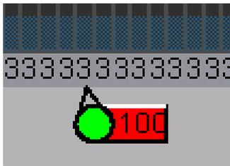
In addition, if there is an alarm on a particular egg diverter, the position indicator turns red.
