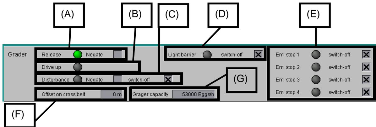
Figure 3-28: Grader “release”
