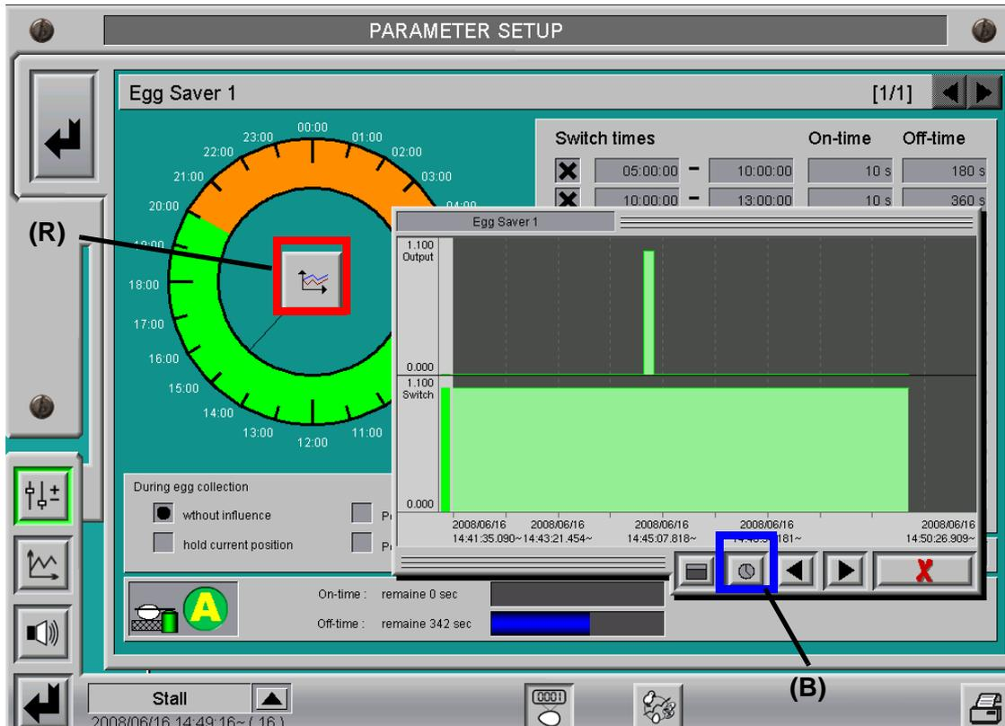
Figure 5-9: Chart of switch times
