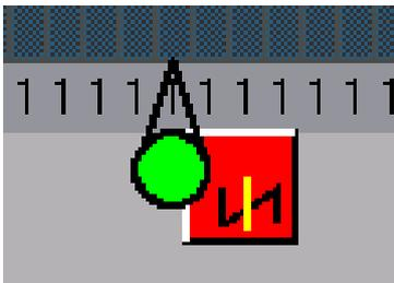
If a chain crack alarm is configured for a belt control, it is displayed as an alarm message. In addition, the alarm for the particular belt control is displayed on the cross belt. The alarm setting is only present in the master control which is responsible for controlling and monitoring the cross belt.
