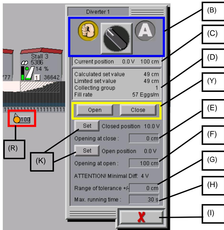
Figure 3-16: Egg diverter in manual mode
