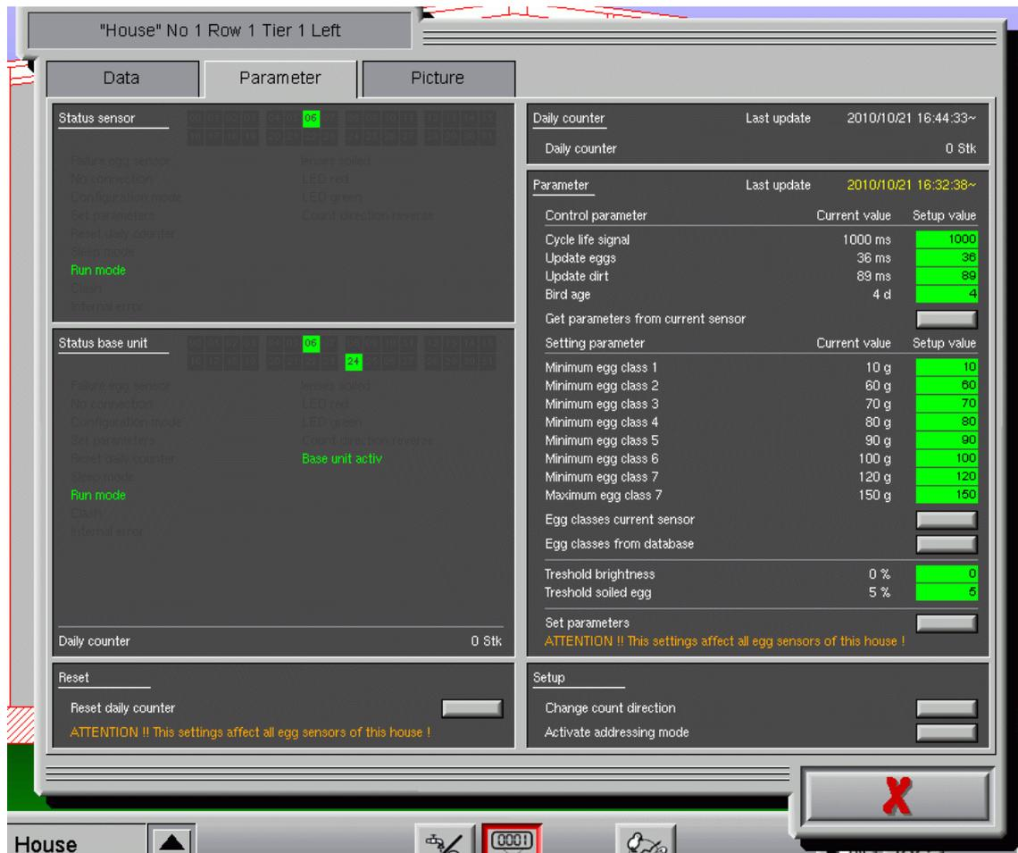
Figure 1-22: OES setting parameters
