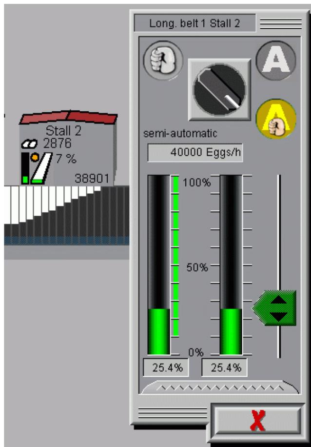
Figure 3-12: Longitudinal belt in semi-automatic mode
