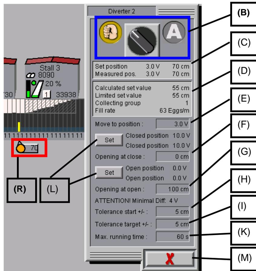
Figure 3-15: Egg diverter II in manual mode
