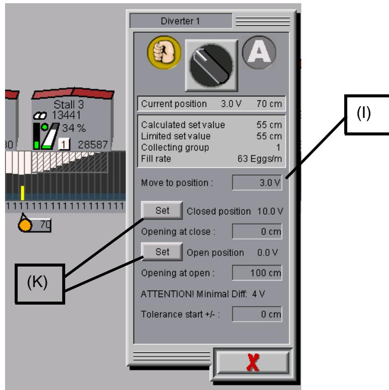
Figure 3-14: Egg diverter in manual mode
