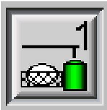
Figure 5-4: "Auto" operating mode, "active", position "up"
