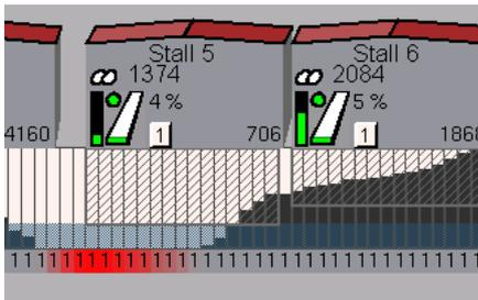
If the fill level of the cross belt exceeds the belt capacity, an alarm is issued. In addition, the congestion on the cross belt is indicated by the area marked in red. **This alarm does not have any influence on the collection process.** Congestion may be caused by manual operating commands, overshooting when starting up the longitudinal belts, etc.
