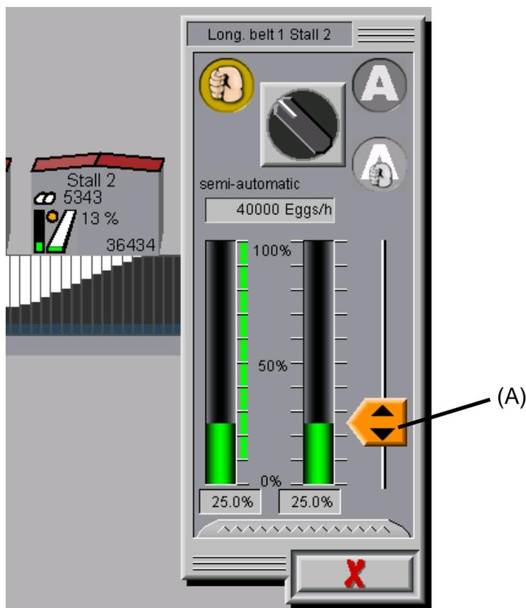
Figure 3-11: Longitudinal belt in manual mode
