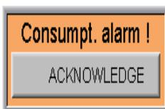
If an alarm is triggered, a control panel for acknowledging this alarm is shown in the main screen. The alarm is reset after it has been acknowledged, and the water valve is opened again if it was closed.
