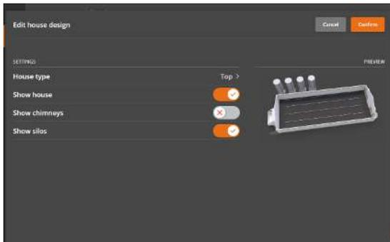
First select the angle of the house illustration. The illustration is shown in the small picture to the right. Then select to hide or display the house, the chimneys and the silos. Finally, save the layout by pressing **Confirm**.
