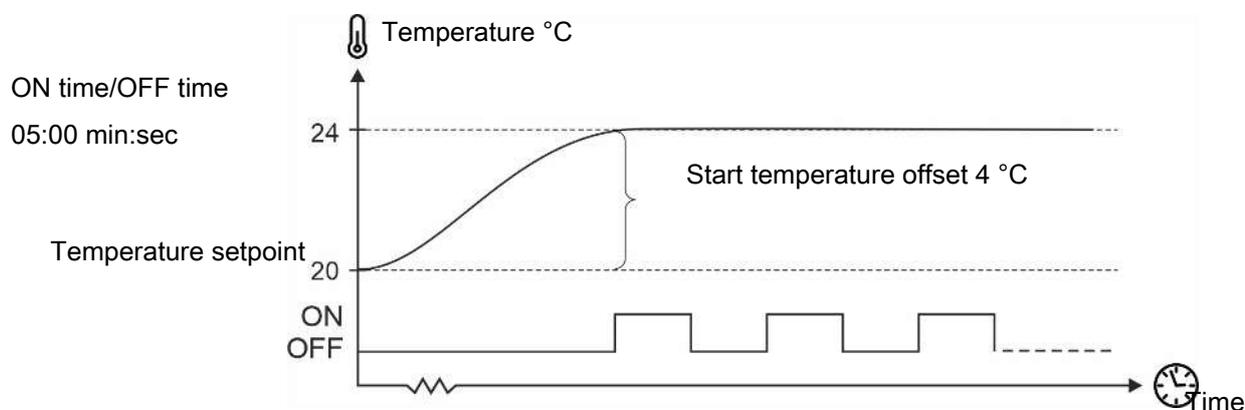
Figure 7: Relay-controlled stir fan (ON/OFF) controlled by temperature
