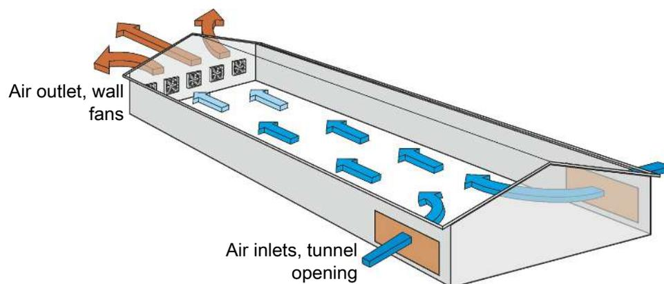
Figure 5: Tunnel ventilation principle
