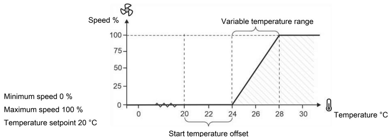
Figure 8: 0-10 V controlled stir fan with a positive Start temperature offset.
