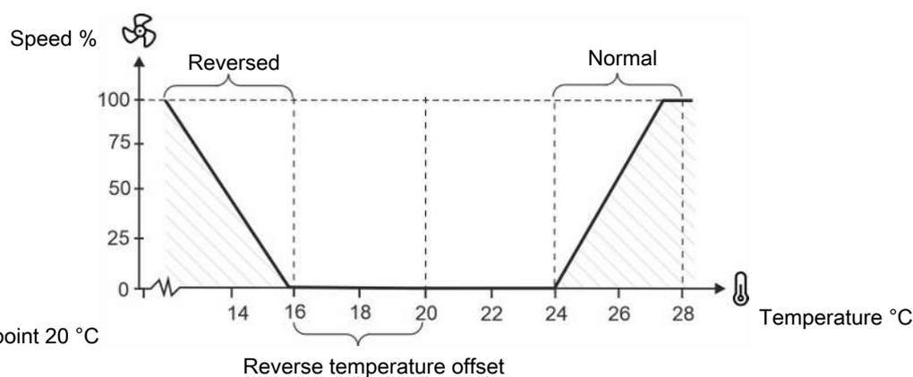
Figure 9: 0-10 V-controlled stir fan with reverse relay
