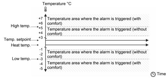
Figure 43: Alarm high and low temperature
