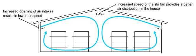
Figure 30: House with free range animals where the ventilation is adjusted at night.
