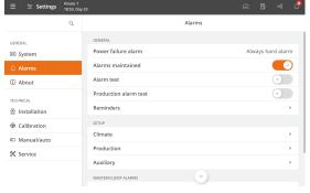
The controller will also trigger an alarm signal, which you can choose to maintain.
