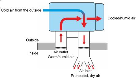
Figure 17: Example of heat recovery unit principle.
