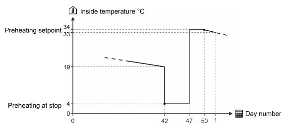
Figure 42: Example of setting of preheating.
