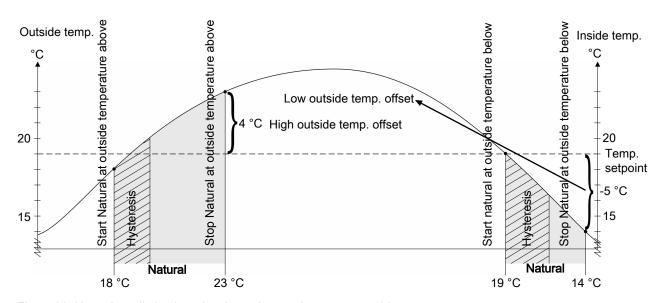
Figure 26: Natural ventilation is active dependent on the current outside temperature.
