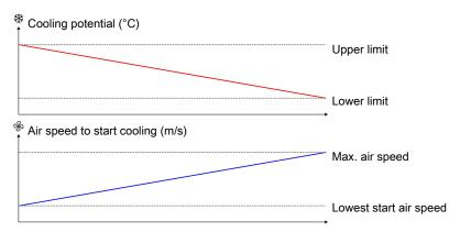
Figure 34: In areas with low outside humidity and a large cooling potential, cooling can start at a lower air speed. Whereas in areas with low cooling potential, cooling will start as late as possible, meaning that it starts at maximum air speed.
