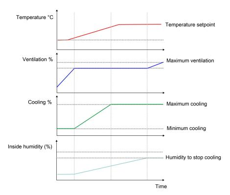
Figure 32: To maintain the required inside temperature, cooling starts before the ventilation level has reached Maximum ventilation. When cooling can no longer maintain the temperature, the ventilation is increased again.
