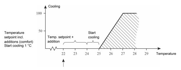
A prerequisite for cooling to be able to start, however, is that ventilation is set to **Maximum ventilation** or that the outside temperature is above **Temperature setpoint**.
