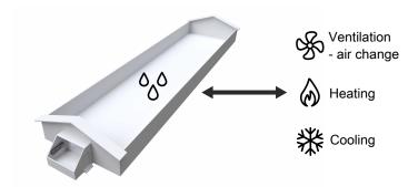
Humidity is supplied to the housing air partly from the animals, feed, drinking water, and animal waste and partly from the cooling and humidification functions.
