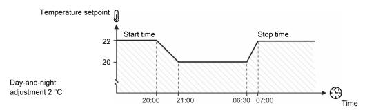
Figure 9: Day and night adjustment set as a nightly lowering of temperature.
