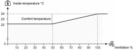
Figure 8: Comfort temperature at continuous production
