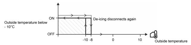
Figure 16: Activation of de-icing
