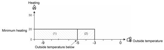
Figure 38: Minimum heat at decreasing or increasing outside temperature
