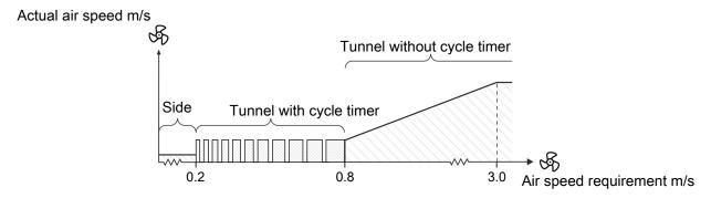
Figure 19: The ventilation sequence with cycle timer at tunnel ventilation
