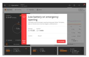
The controller will record the alarm type and time when an alarm occurs.
