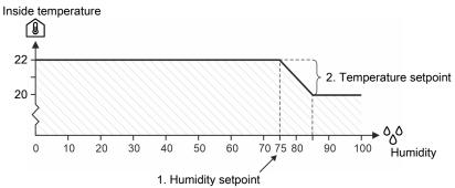
Figure 13: Humidity control with temperature reduction
