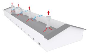
Figure 21: FreeRange ventilation in a equal pressure system
