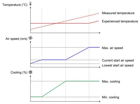
Figure 35: The cooling starts already at low air speed to maintain the required inside temperature. When the cooling cannot maintain the temperature, the air speed is increased again.
