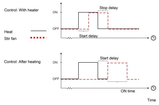
Figure 29: Control with heater
