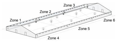
Figure 15: Example of house with zone controlled inlets.
