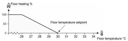
Figure 39: Floor heating with temperature sensor
