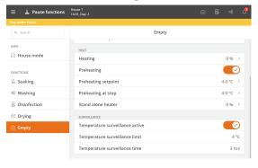
Preheating ensures that the inside temperature does not drop below the set temperature when house status is **Empty** for a longer period of time.
