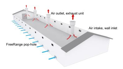
Figure 20: FreeRange ventilation in a negative pressure system
