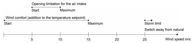
Figure 27: Natural ventilation at increasing wind speeds
