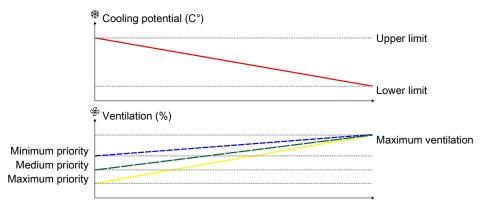
Figure 33: The higher the cooling potential, the higher priority of early cooling start.
