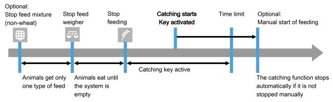
Figure 41: The sequence when stopping the feed system during catching
