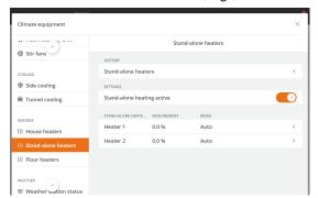
You can use up to 4 stand-alone heaters to which a local zone should be assigned at controller setup.
