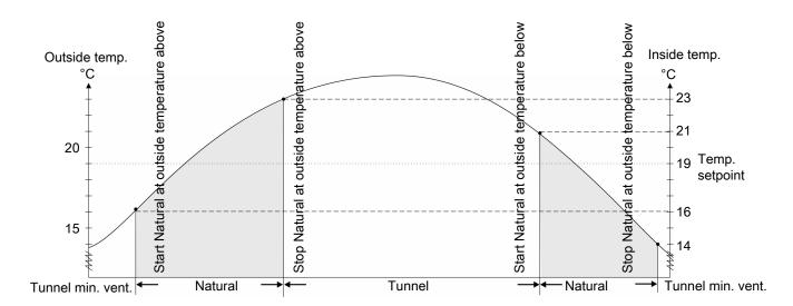
Figure 25: Natural ventilation is active dependent on the current outside temperature. Temperature setpoint is 19 °C.
