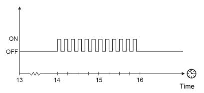
Figure 28: 24-hour clock control
