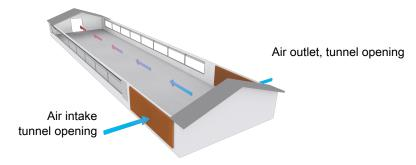
Figure 24: Example of livestock house with natural ventilation in combination with tunnel ventilation, Tunnel ventilation.
