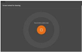
Press Menu button | Settings | General | System | Maintenance | Lock screen for cleaning to lock the screen.
