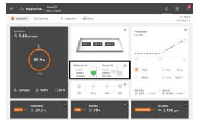
When a silo is shared between several houses, it is regulated by a master controller. Select the master controller and the client controllers during installation.
