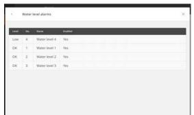
Input terminals in alarm mode are displayed at the top of the list. Next, the faulty input terminals are displayed, which are monitored before an alarm is released. At the bottom of the list, you find the input terminals where the status is OK.
