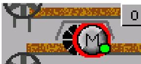
Protective motor protection switch triggered
