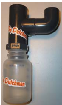
Fig. 2: Measuring cup for flow rate-measurements for nipple drinker
