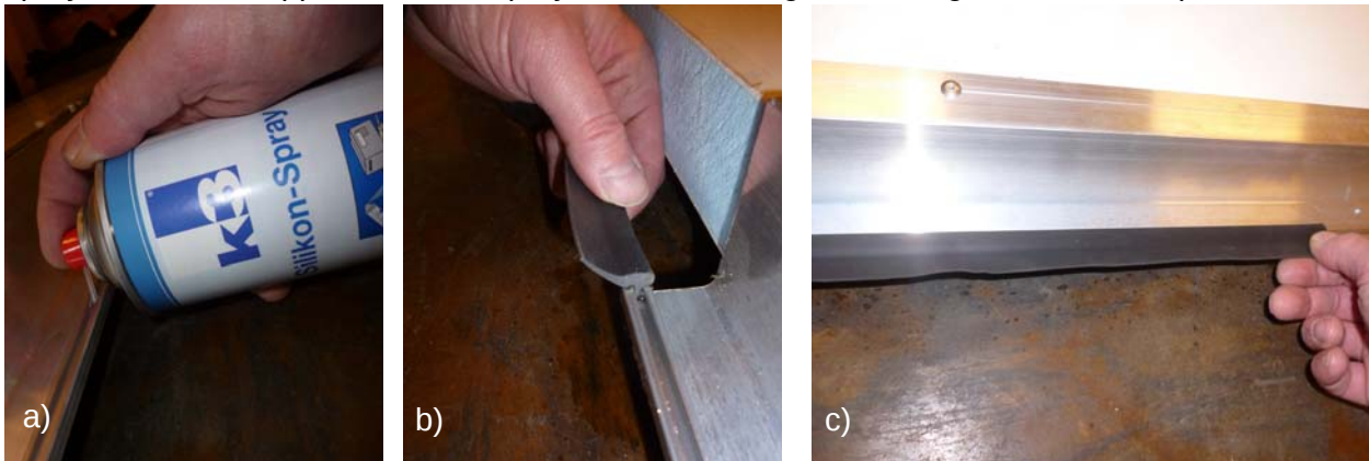
Fig. 2: Inserting the lip sealing (a-c)
