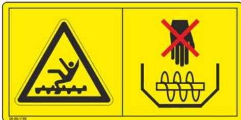
**Danger of drawing-in due to operating auger, chain or rope sheaves!**
