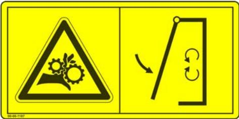
**Danger of crushing due to rotating machine parts!**
