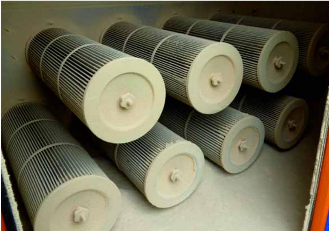
If the temperatures are very low, remove the filters by loosening the star knobs. Blow the filters clean using compressed air or clean them with water.
