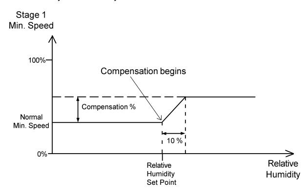
This feature also applies when the minimum ventilation speed curve is activated. Note that for the compensation to take place, the compensation feature must be activated by the user. When a compensation is applied to the minimum speed, the compensation pilot light turns on.
