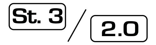
(ii) If, after about 6 seconds, no action is taken by the user, the absolute temperature value is displayed, alternating with "St. 3". In this case, the absolute value is: Set Point + Bandwidth 1 + Offset 2 + Bandwidth 2 + Differential 3.
