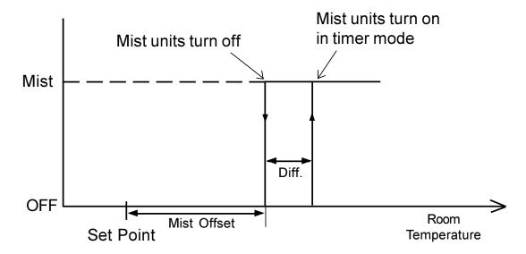
If the humidity compensation is activated, the mist units are turned off when the humidity reaches a user-defined maximum humidity level.
