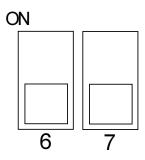
Note that if only one stage is used for heating, it must be Stage 6.
