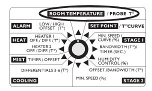
To display the desired temperature, set the selection knob to **ROOM TEMPERATURE**. The readout can display values from -40.0°F to 120.0°F ( -40.0°C to 48.9°C).
