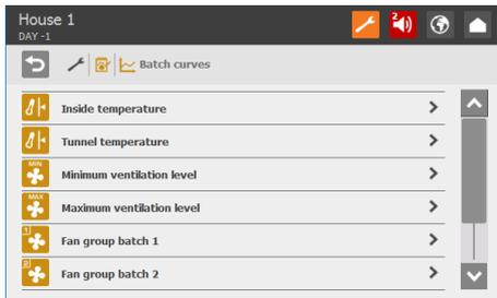
Vento II can automatically adjust settings for temperature, heat, and ventilation.
