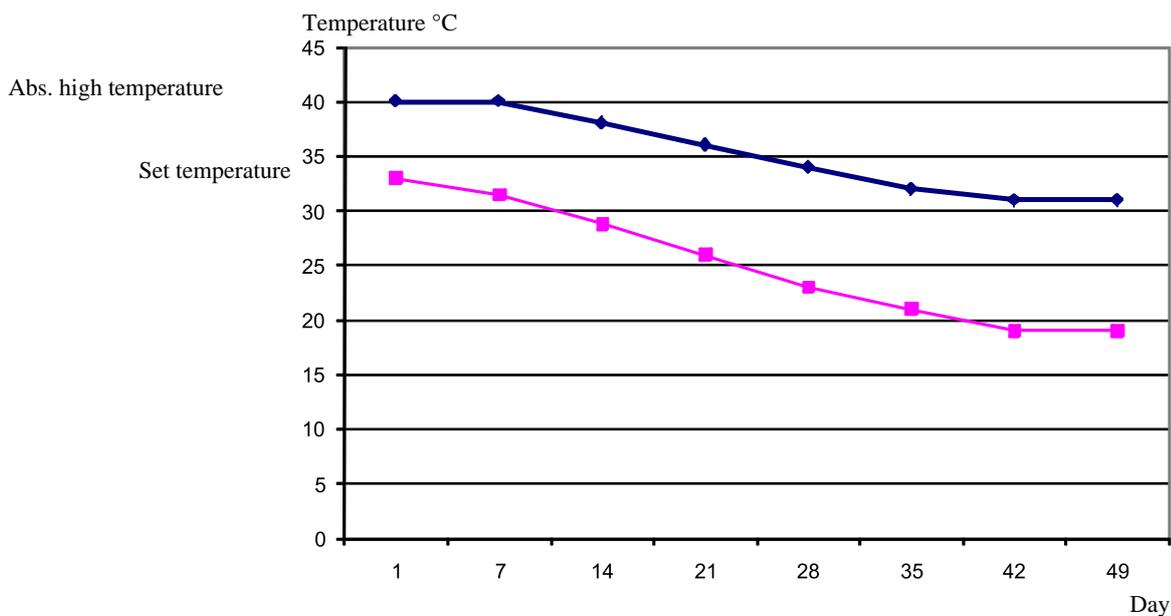
Alarm for Absolute high temperature is released when the inside temperature exceeds the set value. The value can be set as a curve over a time span of eight day numbers.
