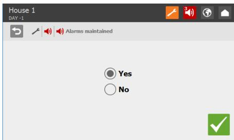
When an alarm occurs, Vento II will register the alarm type and the time it occurred.
