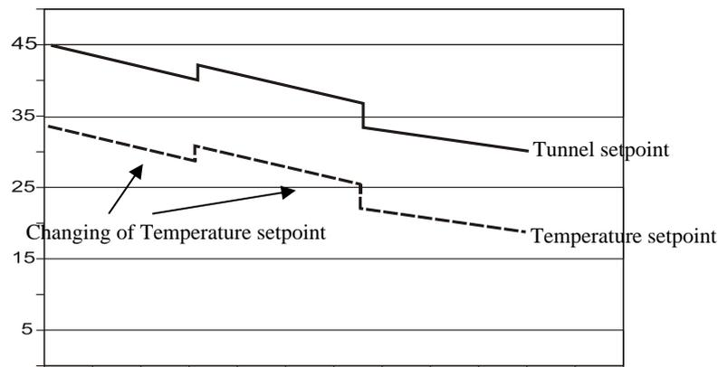
When you change **Temperature setpoint** the Vento II offsets the **Tunnel setpoint** in parallel accordingly.
