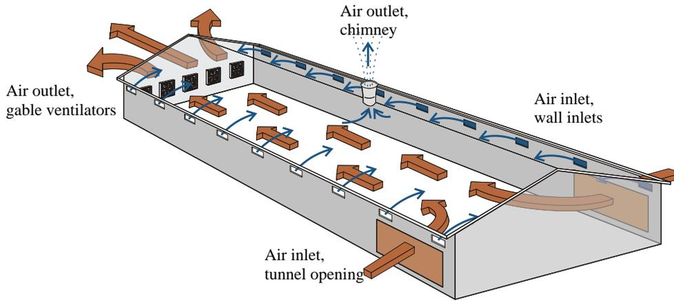
**Figure 1: Combi-Tunnel ventilation**
