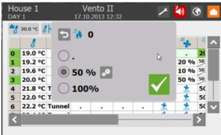
Press a cell to change the settings for the chosen function at this exact level.
