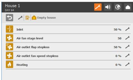
This function will maintain the air change in the house by allowing ventilation to run at a fixed percentage (50%) of the system capacity. This is to protect the animals in case a house is set at **Empty house** by mistake. You can set heating to maintain heat in the house.
