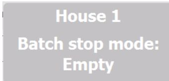
Set batch status to **Active house** the day before stocking the animals so that the climate controller has time to adapt the climate to the animals' requirements. The day number switches to day 0, and the climate controller runs in accordance with the automatic climate setpoints.
