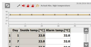
The absolute high temperature alarm is set as a temperature curve.
