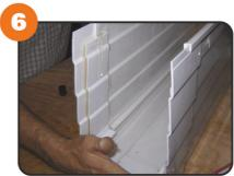
5. The Tangit adhesive should **ooze out of the gap** when joining the components. If this does not happen, you did not use sufficient adhesive.
