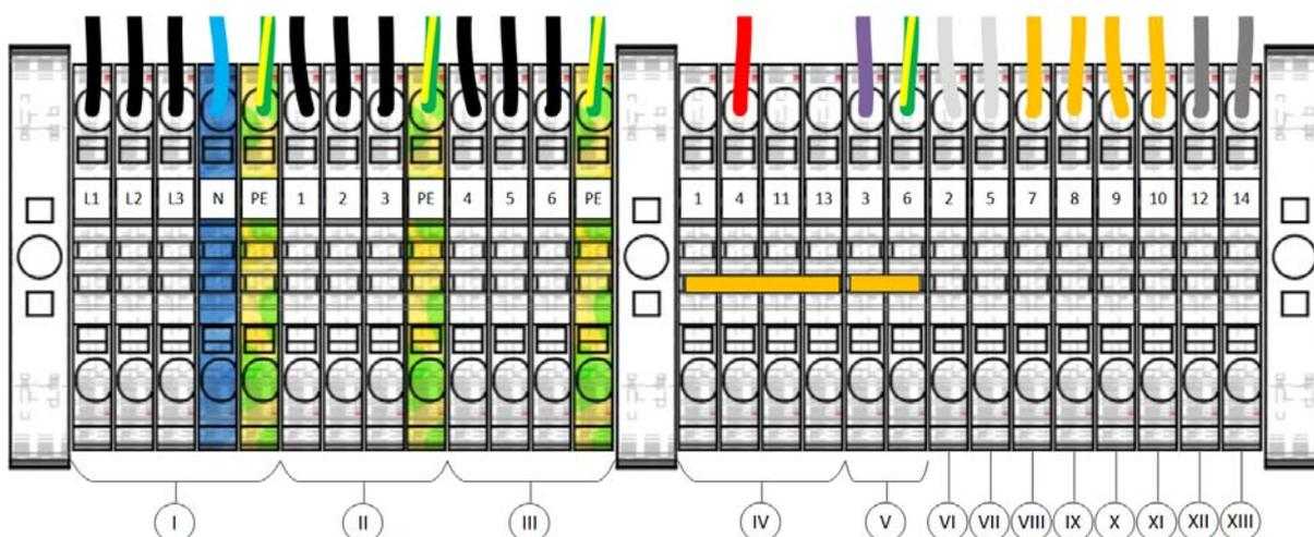
Figure 4-2: Terminal strips – version for two circuits
