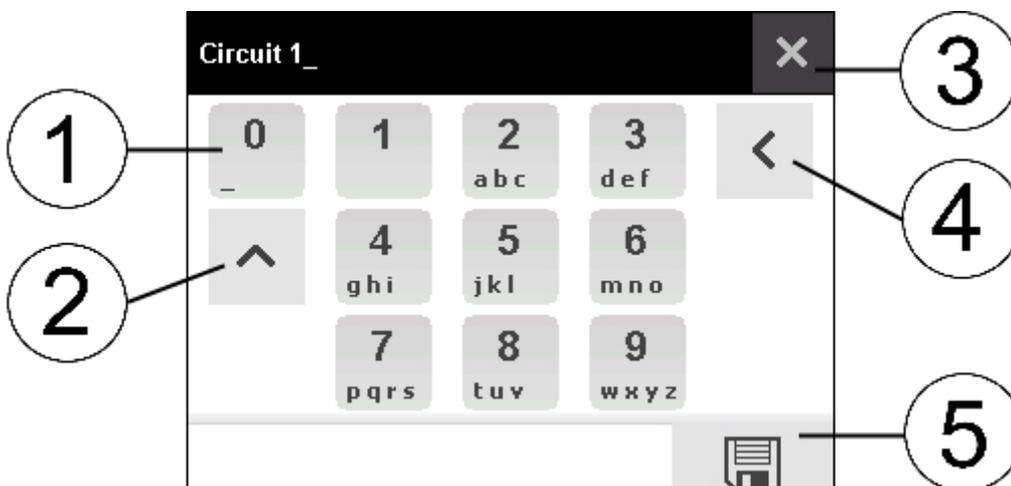
Figure 5-11: Changing the name of a feed circuit
