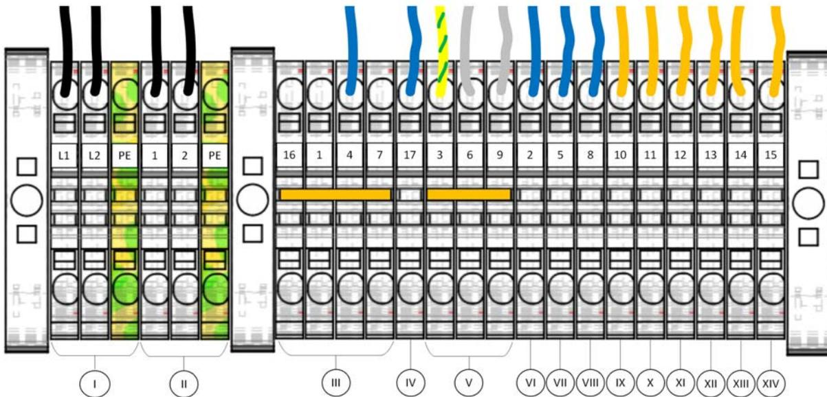
Figure 4-3: Terminal strips – version for one circuit (US version)
