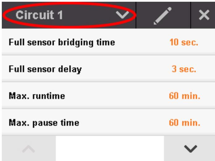
Figure 5-10: Selected feed circuit
