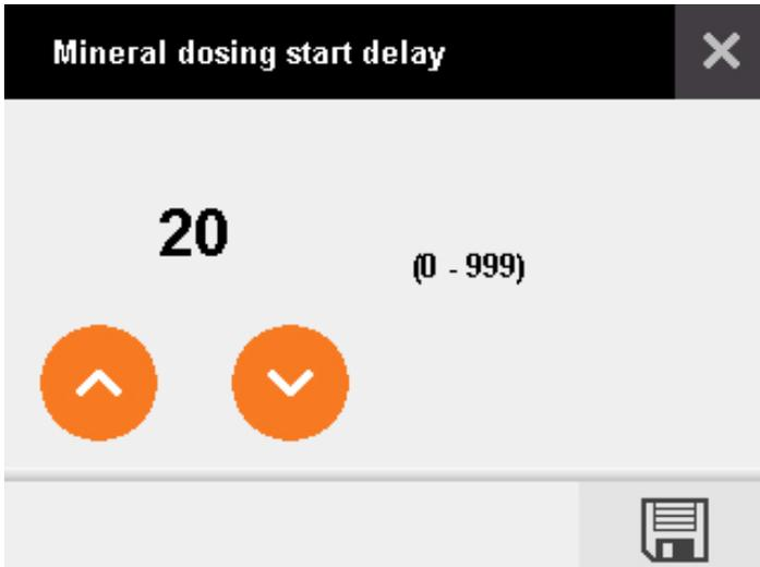
Figure 5-17: Start delay of the mineral dosing unit
