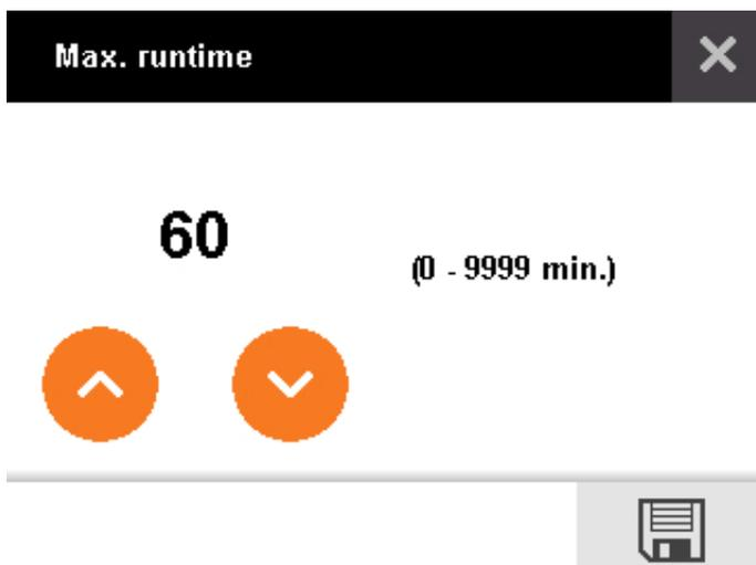
Figure 5-14: Maximum runtime of the feeding system
