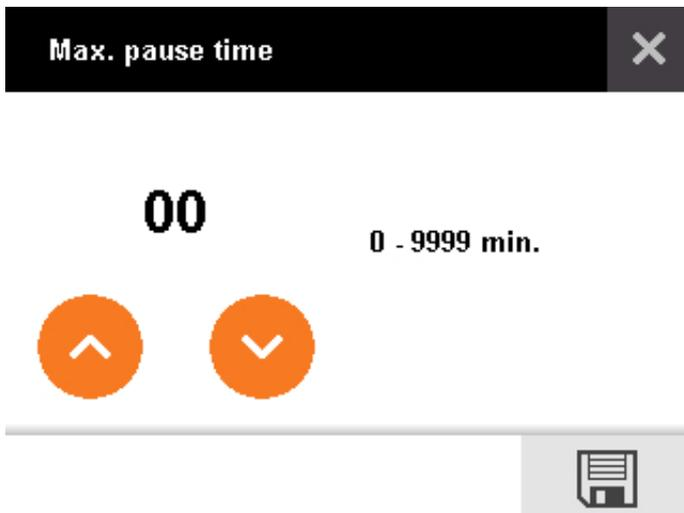
Figure 5-15: Maximum pause time of the feed circuit
