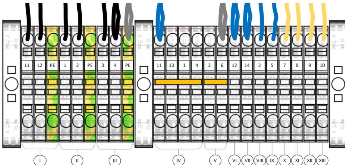
Figure 4-4: Terminal strips – version for two circuits (US version)
