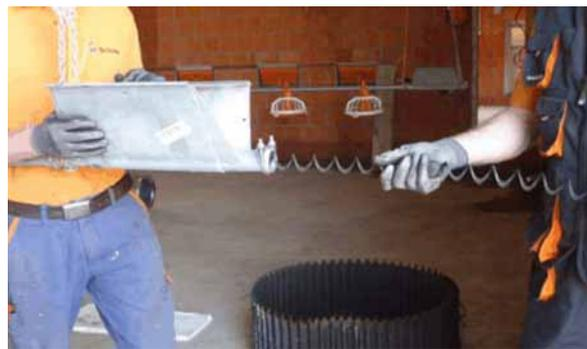
Figure 6-8: Insert the auger
