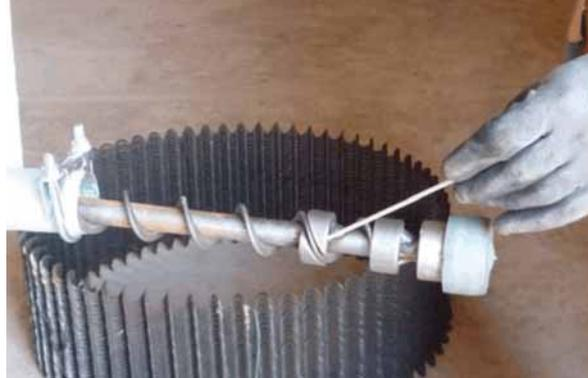
Figure 6-18: Fix auger
