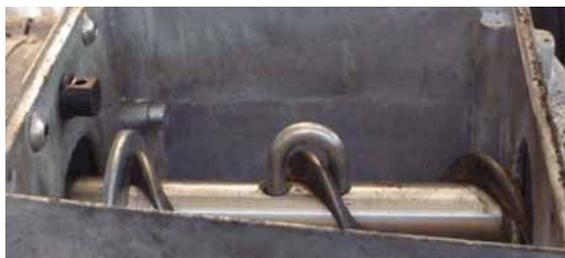
Figure 6-9: Fix the auger to the drive
