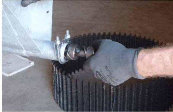
Figure 6-23: Pull out tension shaft
