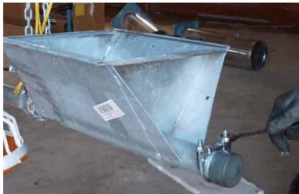
Figure 6-20: Fasten the tension shaft
