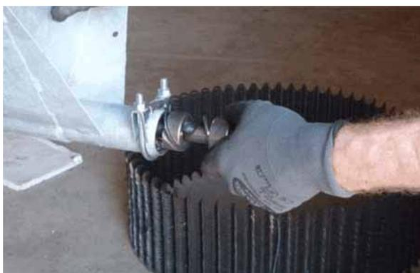
Figure 6-28: Hold the tension shaft
