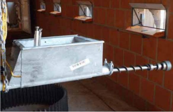
Figure 6-17: Auger to tension shaft
