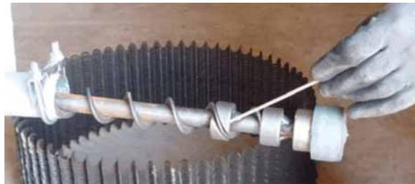
Figure 6-25: Loosen the auger from the tension shaft
