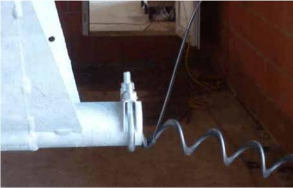
As soon as the auger has its natural tension, it is marked at the outlet of the *lower part for feed hopper* (for example by means of a cable strap Figure figure 6-11).
