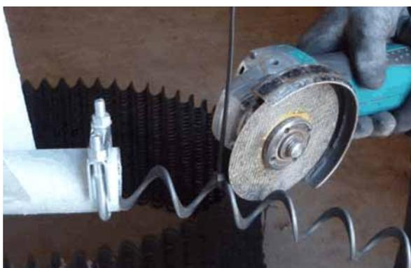
Figure 6-15: Cut off auger
