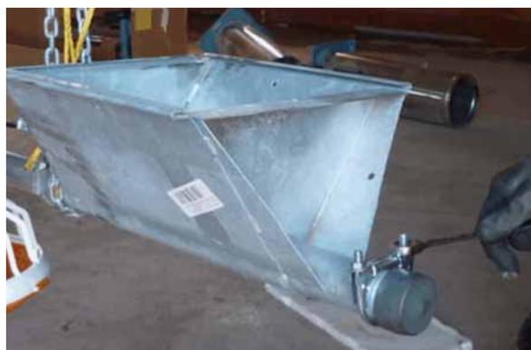
Figure 6-29: Fasten the tension shaft
