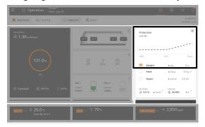
Operation. A graphic on the Production results card shows the current average weight for the last 48 hours (14 days for breeder).
