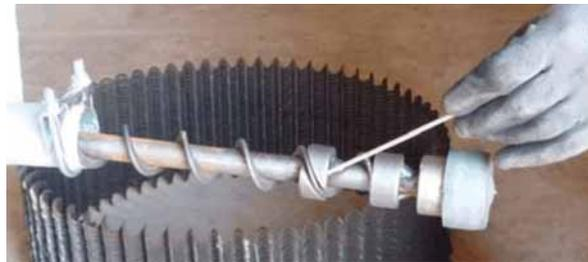
Figure 5-5: Loosen the auger from the tension shaft
