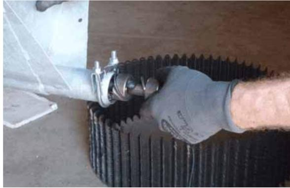
Figure 5-3: Pull out tension shaft
