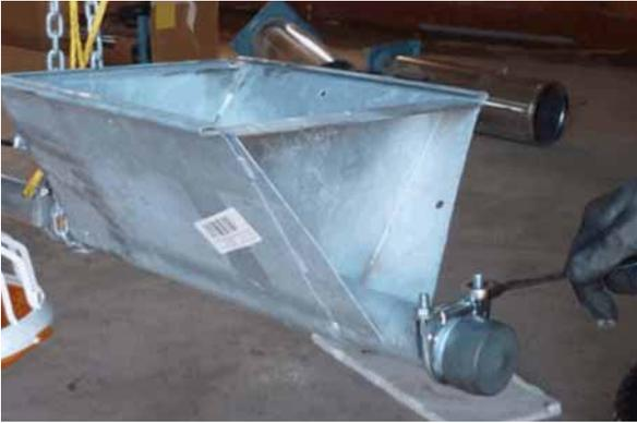
Figure 5-2: Loosen U-bolt
