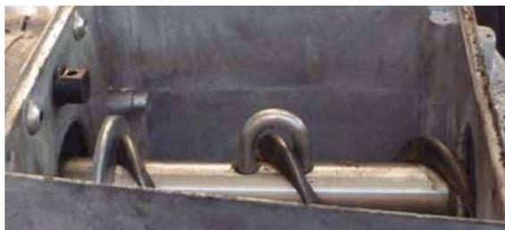
Turn the auger up to the guard plate for drive shaft and clamp the auger by means of the hooked bolt.
