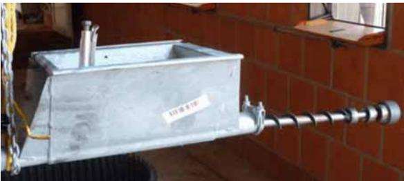
Figure 5-4: Fix the auger by means of a vis-grip wrench
