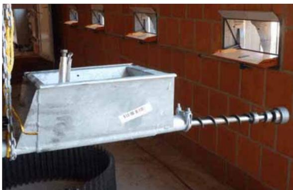
Figure 5-6: Auger to tension shaft
