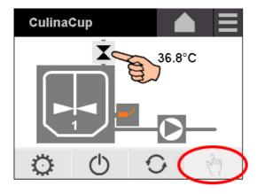
2. Press the button for the water valve until the window **Manual dosing time water** opens.
