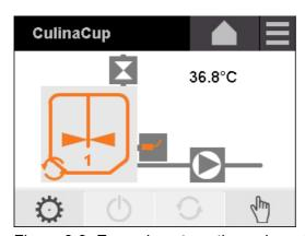
Figure 6-8: Example automatic mode: agitator active
