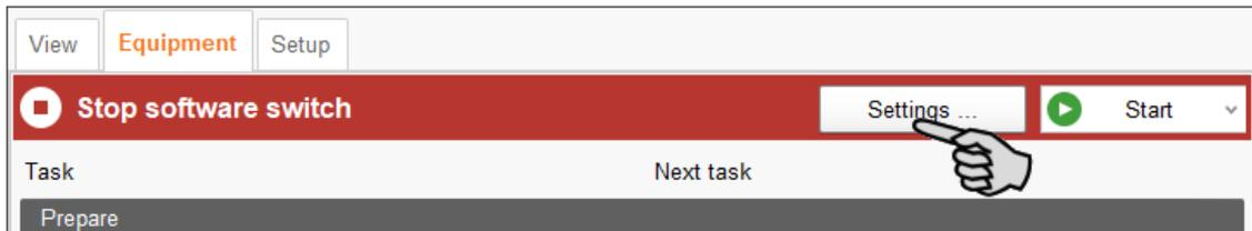
This opens the settings dialog, which contains all settings for the system components you defined in the Composer beforehand. The settings are grouped and may have pre-set values. The different parameters are described in the following chapters.
